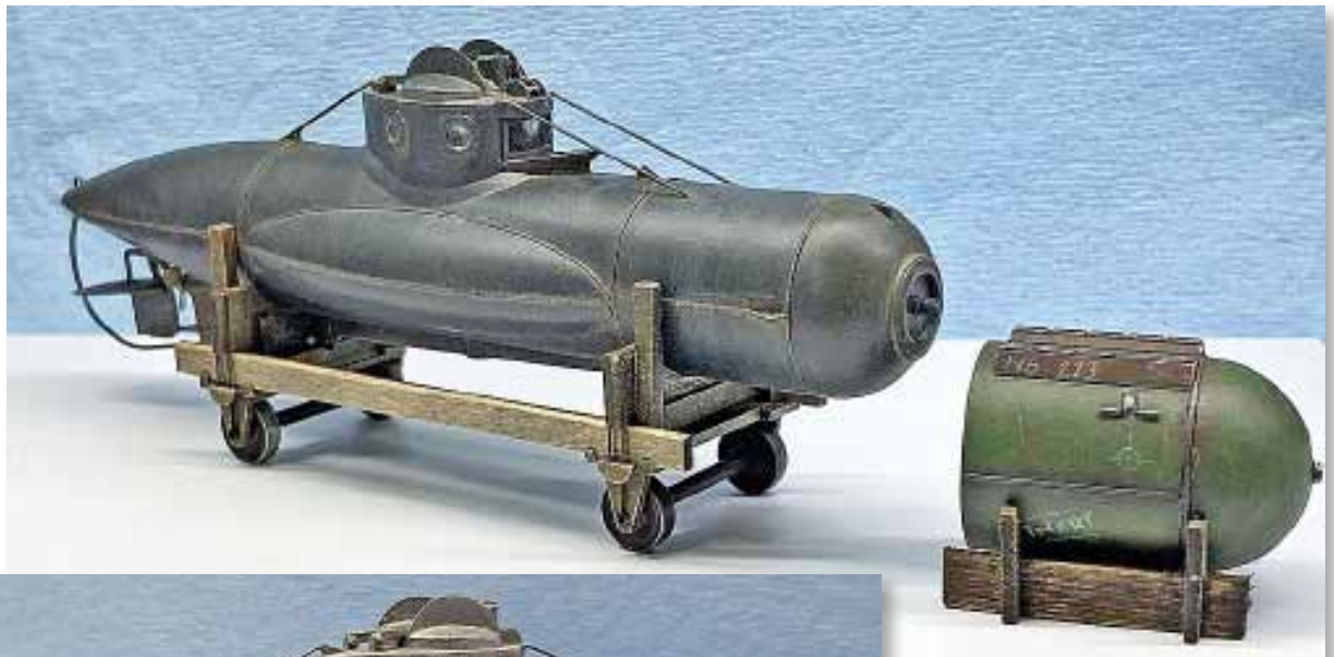
Two views of the completed Welman W10 on its transport cradle, with detached explosive charge.
