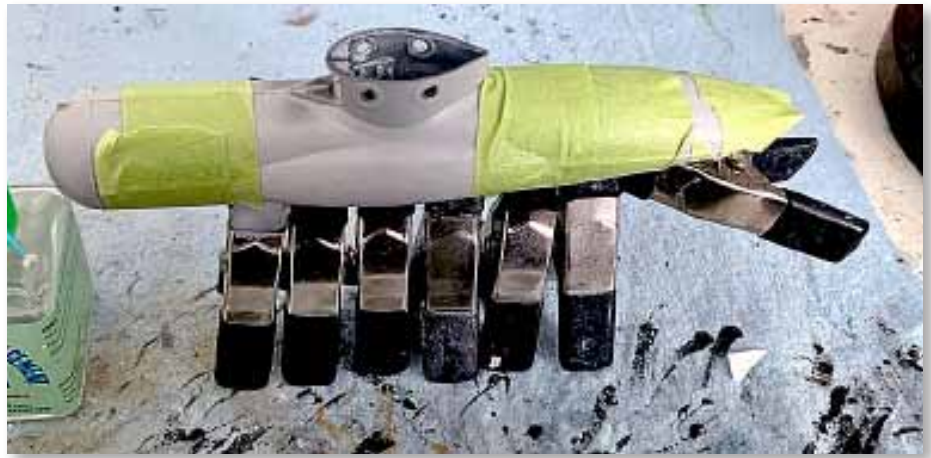
Strong measures used to bind and clamp the assembled hull
